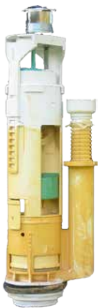
Scale deposits in the complex design may cause leaks.
